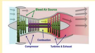
**Figure:** shows air entering the front of the engine where a series of turbines compress, warm and pressurize the air before it passes into the combustion chamber where it is ignited to create the airplane's thrust. This "bleed" air is drawn out of the engine into the cabin after it is pressurized, but before the combustion chamber.
